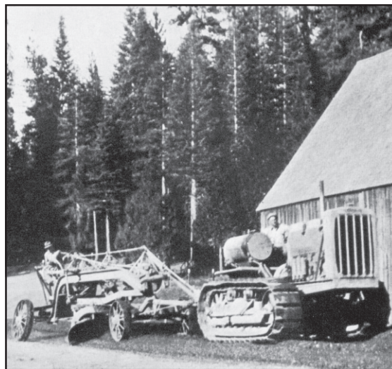
Caterpillar Diesel Tractor No. 1. Built in 1931, this was the first diesel Caterpillar Tractor. In this picture, taken between 1931 and 1936, it is pulling a “blade grader.” (Reproduced from Caterpillar Tractor Company n.d.; courtesy Dave Smith, Secretary/Treasurer, Antique Caterpillar Machinery Owners Club.)
